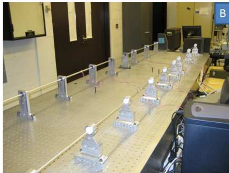
Figure 3.5: (A) A schematic of a split-Hopkinson pressure bar apparatus[11].(B) A photograph of an in-house built aluminum split-Hopkinson pressure bar apparatus.
