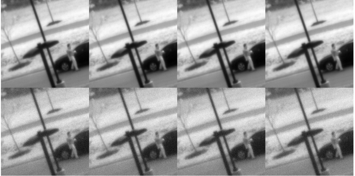
Figure 2.1: Noisy and blurred polarimetric imagery. The First row has an SNR of 25dB and the second row has an SNR of 15dB. From left to right the angle of the polarizer is \{0^\circ, 45^\circ, 90^\circ, 135^\circ\}
