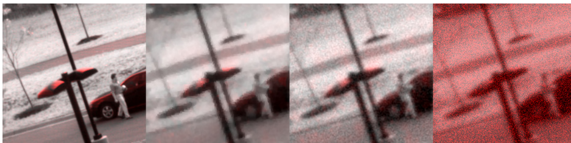
Figure 3.10: Image estimation results for \text{SNR} = 25\text{dB} . From left to right: object, estimate using edge-preserving regularizer, estimate using quadratic regularizer, and the conventional estimate.
