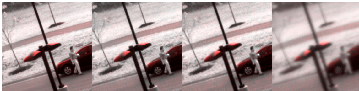
Figure 3.9: Image estimation results for \text{SNR} = 45\text{dB} . From left to right: object, estimate using edge-preserving regularizer, estimate using quadratic regularizer, and the conventional estimate.
