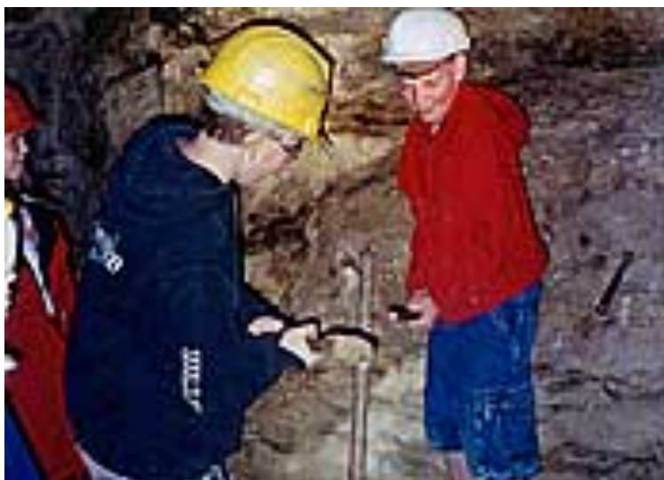
Photo 11.6: Double jacking at the Phoenix mines, Courtesy of Clear Creek Watershed Foundation.
