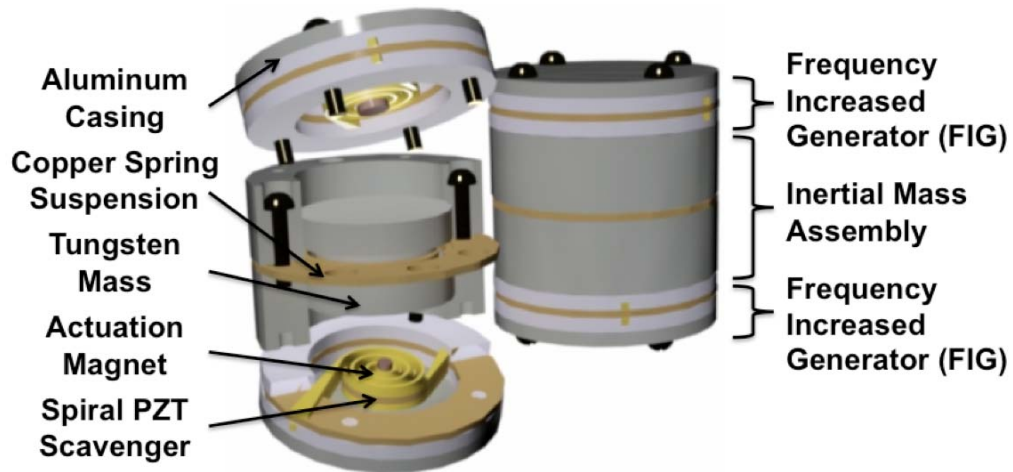
Figure 4-1. Rendering of the piezoelectric PFIG, showing the layout and the different components.
