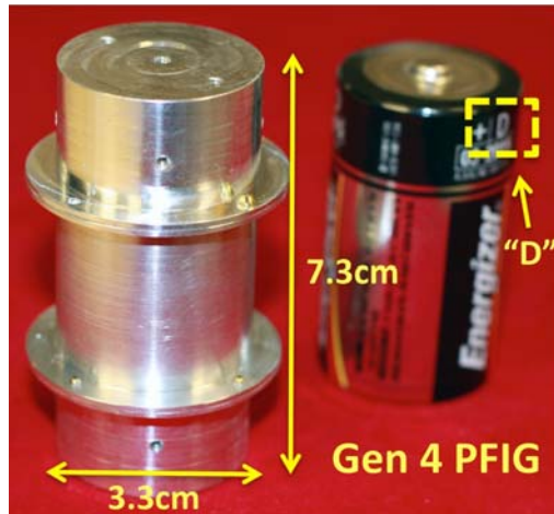
Figure 5-14. Photograph of the completed Gen 4 PFIG alongside a “D” size battery.
