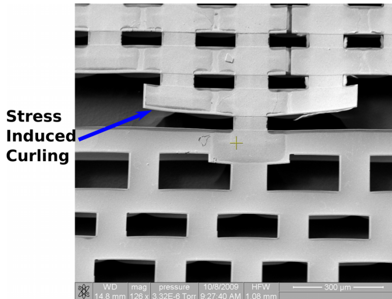
Figure 5.8: An SEM image of the inter-stage zone between stages 2 and 3 of a 4-stage cooler. The zone is not supported by any oxide pillars, and curling of the inter-stage zone is clearly visible. This is in contrast to Figure 5.7, which shows very little deflection of the interstage zones where they are supported by the pillars.
