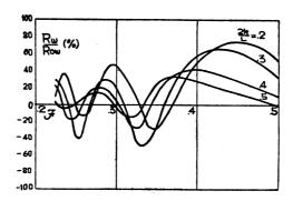
Fig. 10. Interference term against Froude number for T/L=0. (Reproduced from Fig. 3, Ref. 7. 2k/L and  $K_{\rm O}$  in the figure corresponds to k and  $2K_{\rm O}$  in the present paper, respectively.)
