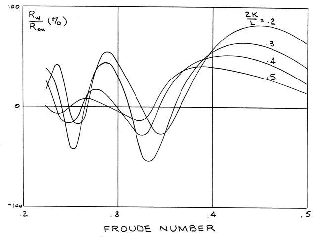
Fig. 9. Interference term plotted against Froude number for T/L=0. (Reproduced from Fig. 5, Ref. 6. 2k/L and  $K_O$  in the figure corresponds to k and  $2K_O$  in the present paper, respectively.)
