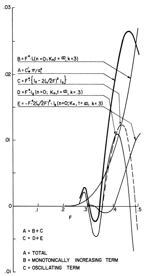
Fig. 5. Contribution of  $I_1$ ,  $I_2$ , and  $I_3$  to the resistance increase due to interference for a given distance between two hulls.
