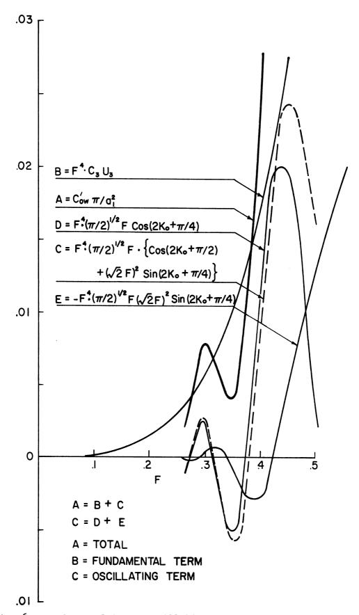
Fig. 6. Fundamental term, oscillating term, and total wave-making resistance coefficient of each hull.
