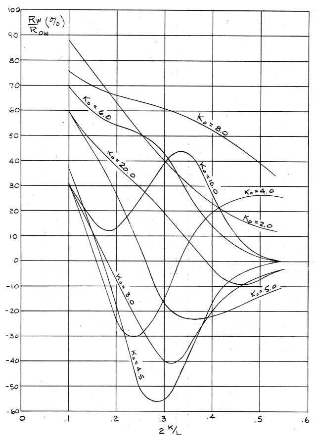
Fig. 8. Interference term plotted against the distance parameter 2k/L. (Reproduced from Fig. 4, Ref. 6. 2k/L and  $K_O$  in the figure corresponds to k and  $2K_O$  in the present paper, respectively.)
