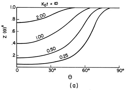
Fig. 7(a). Factor representing the draft effect:  $Z^2(\theta) = (1-e^{-K_0 t} \sec \theta)^2$ .
