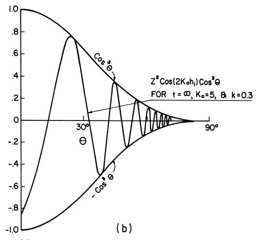
Fig. 7(b). Integrand of one of the oscillating terms, i.e., I21.
