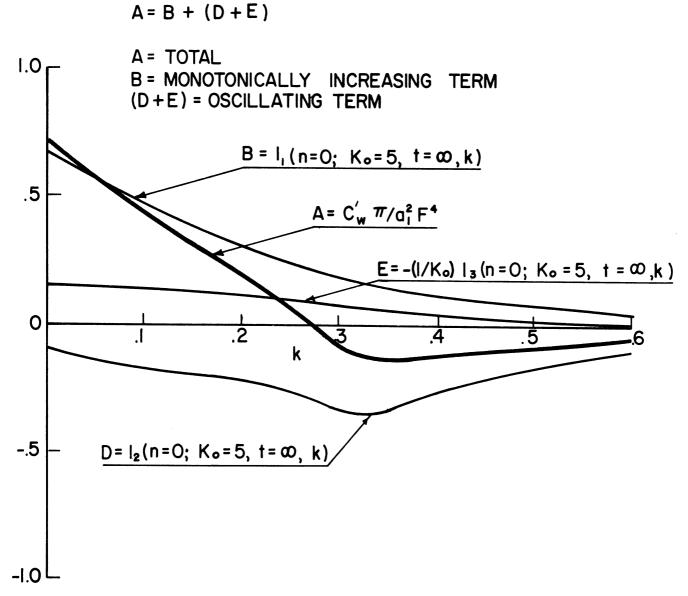
Fig. 3. Contribution of  $I_1$ ,  $I_2$ , and  $I_3$  to the resistance increase due to interference for a given advance speed.
