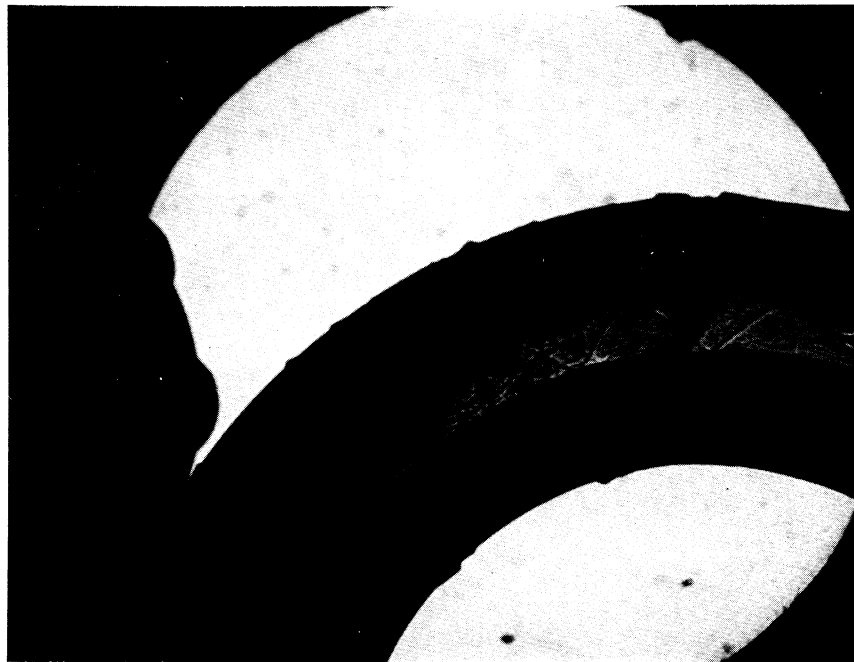
Fig. 14. Spark-schlieren photographs at different magnifications of two 60%, H_2-O_2 detonation waves passing through the curved test section.
