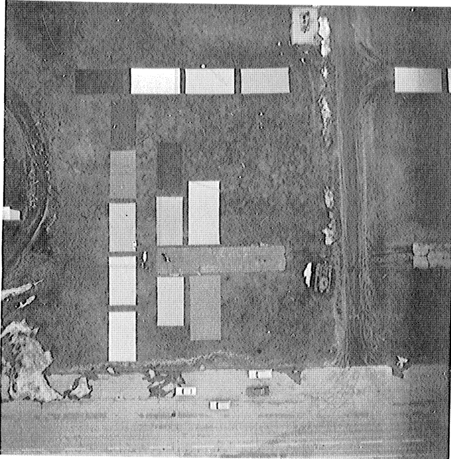
FIGURE A-7. IMAGERY OF REFERENCE PANELS. Panels on Willow Run Airport ramp, 3/15/67, 1156, altitude 500 ft., with Ansco D-200 film using a 1A filter.
