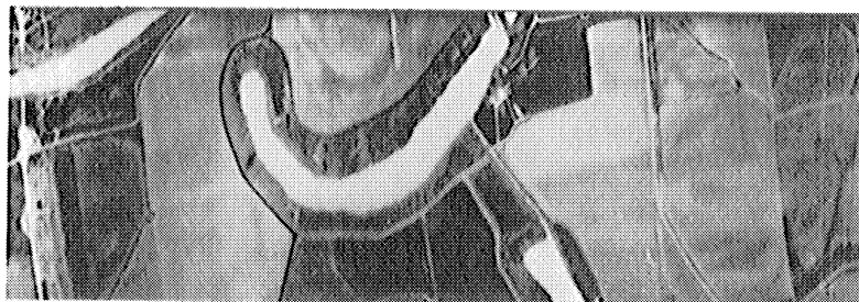
FIGURE 2-10. THERMAL IMAGE OF AN AGRICULTURAL SCENE, 8-13 MICRONS
