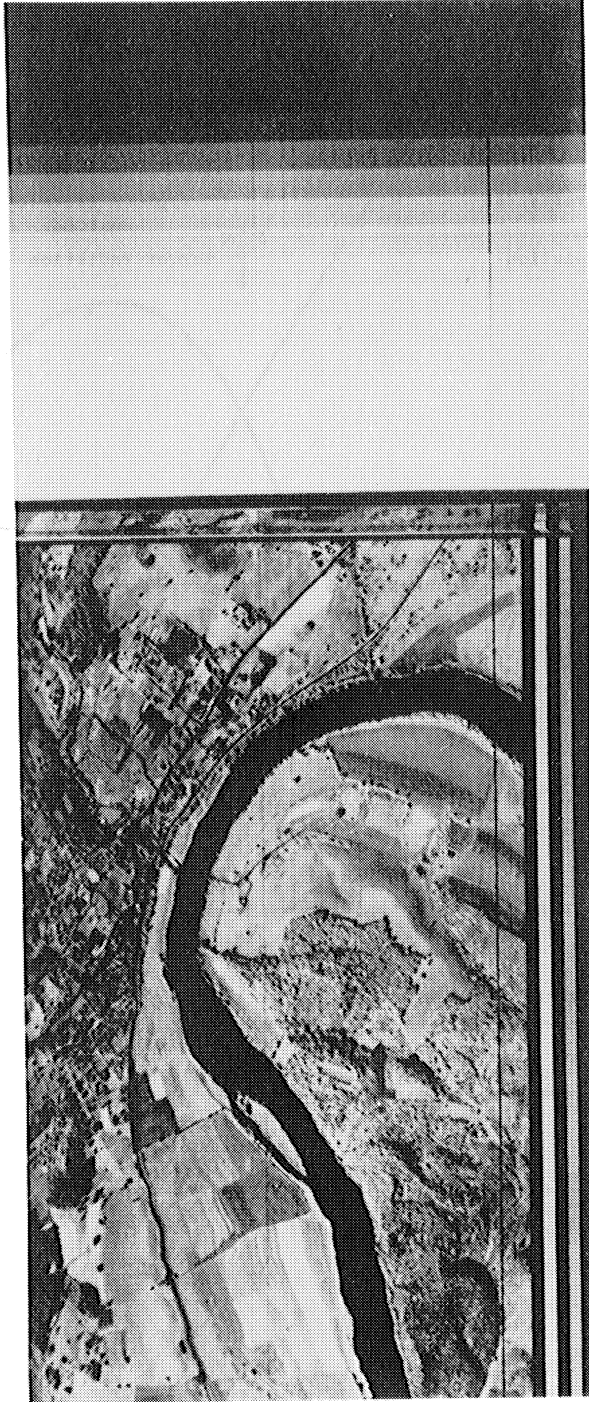
FIGURE A-2. TYPICAL IMAGERY WITH REFERENCES AND GREY SCALE PRINTOUT. Holston River at Sargoinville, Tenn., 9/3/67, 1643, altitude 4000 ft., 0.8 to 1.0 micron imagery by University of Michigan, IST, IROS.
