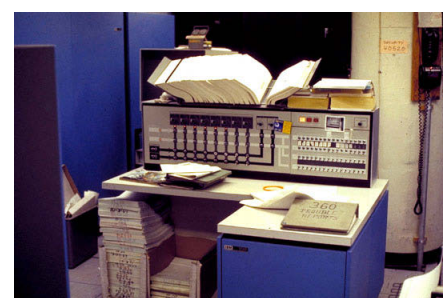
2167 configuration console for the IBM System/360 Model 67-2 (duplex) at the University of Michigan, c. 1969
