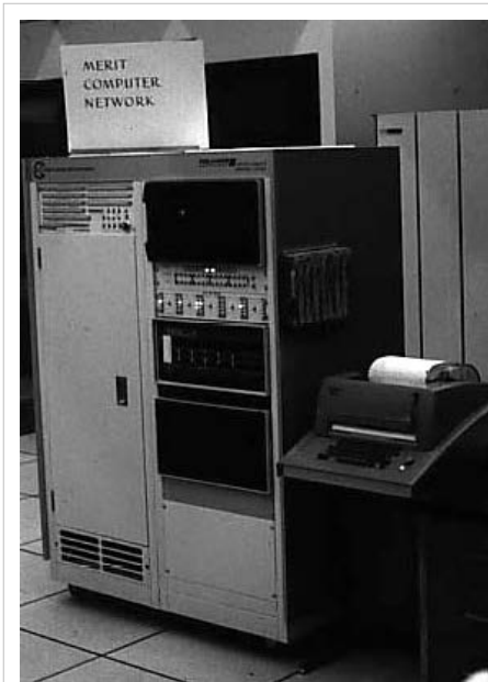
Merit PDP-11 based Primary Communications Processor (PCP) at the University of Michigan, c. 1975
