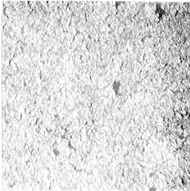
Figure 16.-- Photomicrograph of silver bromide crystals in collodion auto-radiographic emulsion. Polarized illumination. Collodion type AW. 1-hour exposure. 1,000X.
