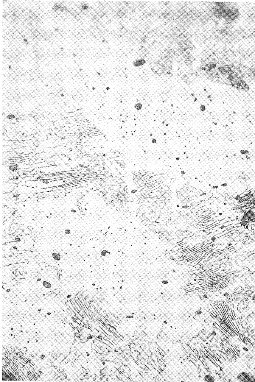
(a) Bare metal, picral etch. 500X. L-84834
