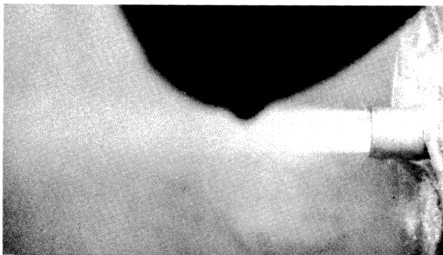
Figure 39. G = 1.38 \times 10^5 lb/hr ft 2 , \chi_e = 47\% , q/A = 200,000 Btu/hr ft 2 , W = 290 lb/hr
