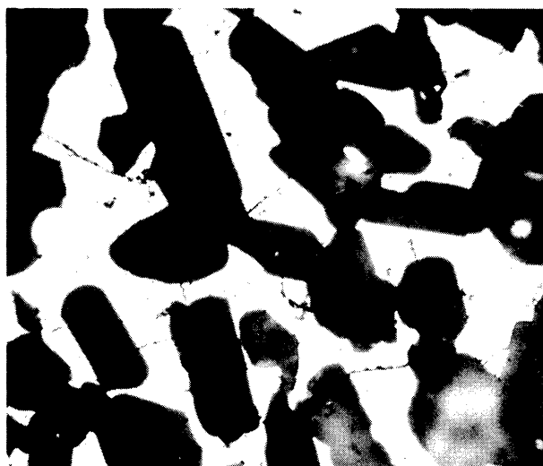
(b) Preheated 18 hours at 2600°F, then 2 hours at 2700°F in air.
