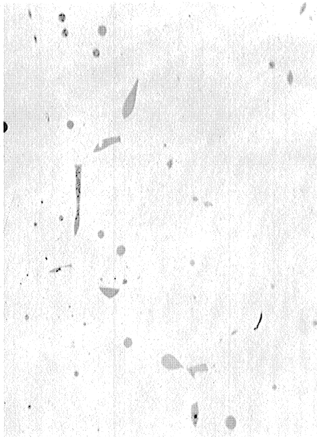
(c) 0.3% oxygen added (inclusion angle - 54^\circ ).
