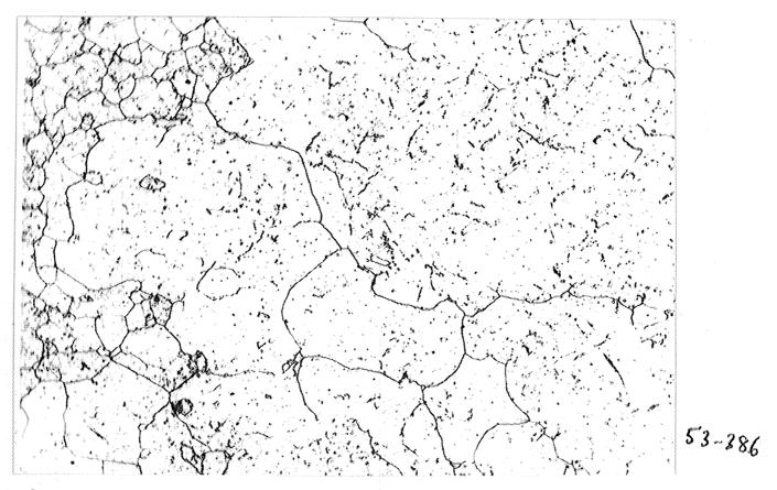
a. One per cent cold reduction before final heat treatment. The finer grain shown in the upper left was found at the center of the bar as rolled.
