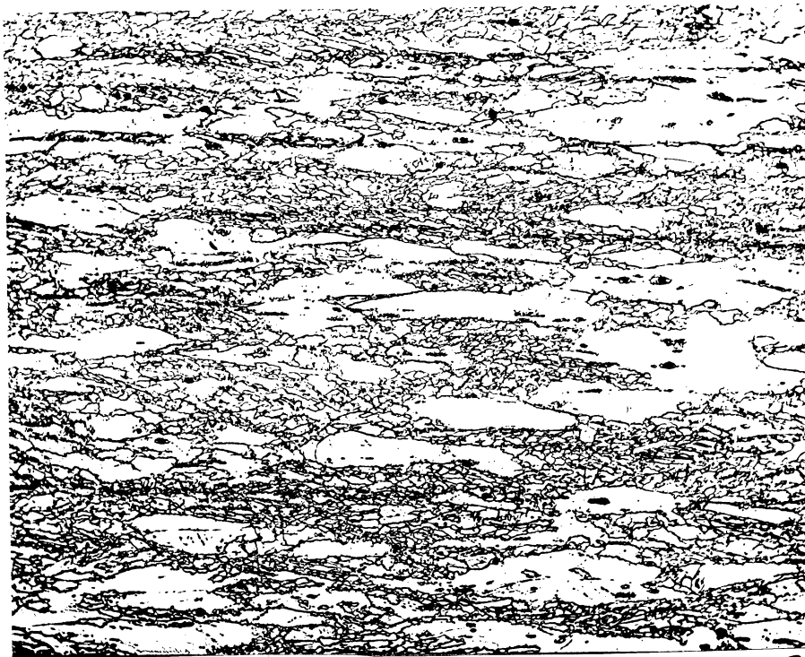
(b) As-Removed from Service Plus 1057 Hours at 1200°F Under 20,000 psi - X100D 62-008
