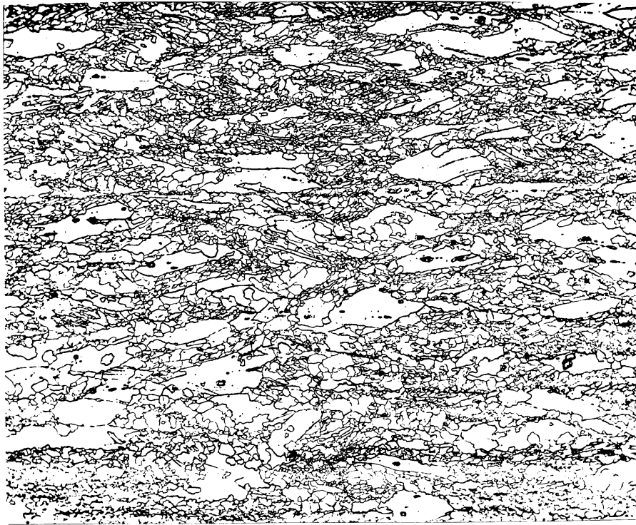
(a) As-Removed from Service - X100D 62-007
