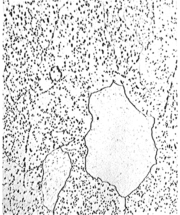
(b) Simulated 10,000 Hrs. at 1100°F
