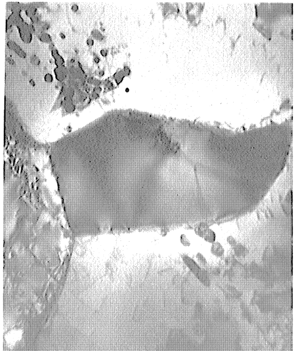
Figure 17: Transmission Electron Micrographs of Type 304 Steel, Cold Reduced 40 Percent and Exposed 100 Hours at 1350°F. X 20,000
