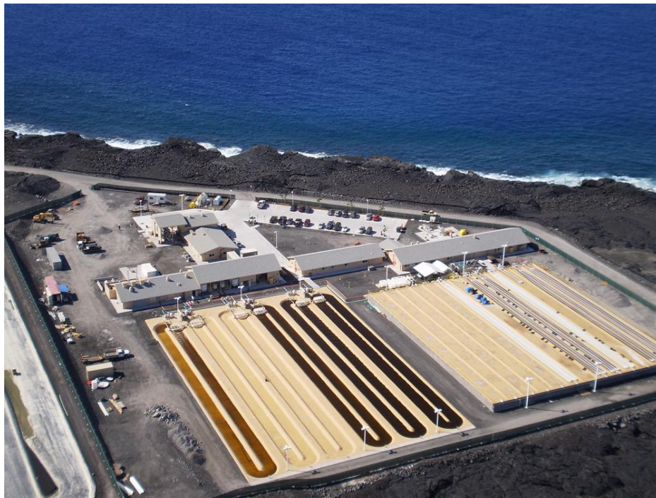
Figure 2. Aerial photograph of a pilot facility operated by HR BioPetroleum-Cellana, Hawaii. Autotrophic microalgae cultivated in open pond raceways using seawater. (Cellana, 2011)
