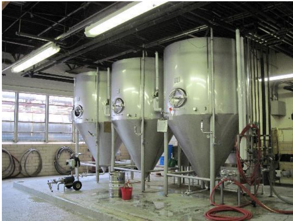
Figure 3. Photograph of three fermenters (bioreactors ) that are likely to be used in System B for the cultivation of heterotrophic algae Chlorella protothecoides . (topmachinebiz.com, 2011)
