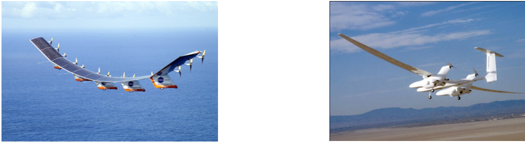
Figure 1. Aerovironment's Helios (left) and Aurora Flight Sciences' Theseus (right) showing large wing deflections (Courtesy NASA Dryden)
