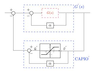
Figure 17. CAPIO  $\in [\alpha,\beta]$  transformed to CAPIO $_t \in [0,\beta-\alpha]$  via loop transformation.
