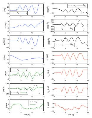
Figure 8. Pitch and roll angles  $\theta$  and  $\phi$ , aircraft states x, on the left. Desired (commanded) and actual attitude accelerations v and Bu, and the control surface deflections  $\delta$ , on the right, when a conventional control allocator is used.
