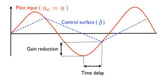
Figure 2. Input u and output  $\delta$  of a rate saturated actuator.
