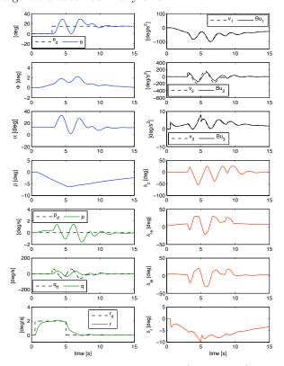
Figure 9. Pitch angle  $\theta$  and aircraft states x, on the left. Desired (commanded) and actual attitude accelerations v and Bu, and the control surface deflections  $\delta$ , on the right, when CAPIO is used.
