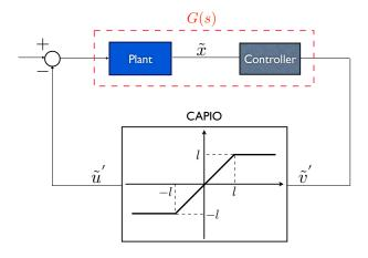
Figure 14. Closed loop system with CAPIO, reconfigured.
