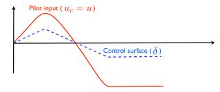
Figure 5. Bias caused by the differentiate-limit-integrate approach
