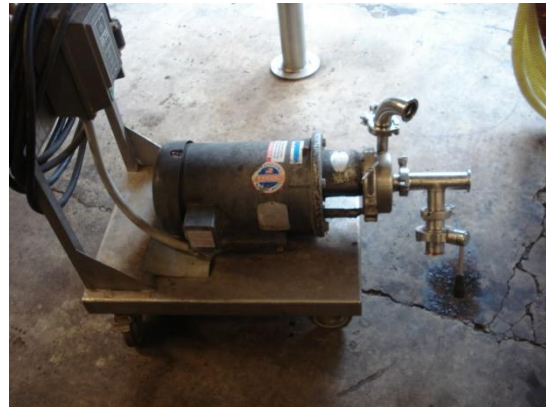
Figure 39 Clean In Place (CIP) cleaning pump
