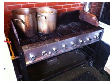
Figure 28. Inefficient use of heating surface
