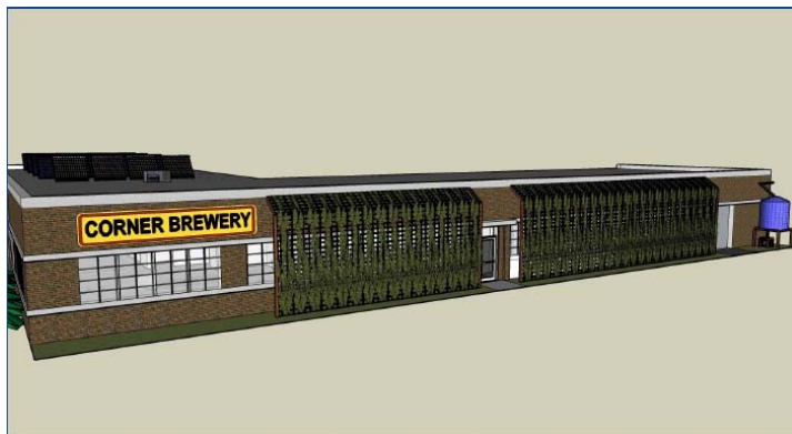
Figure 55. The hop wall offers superb shading in the summer, while providing a key ingredient used for small batches
