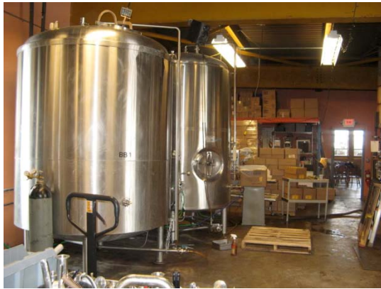
Figure 38 Bright tanks in the brewhouse
