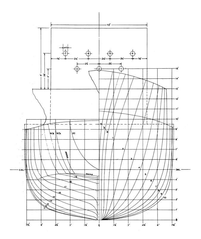
Figure 2. View of Destroyer Model Showing Deckhouse Configuration and Location
