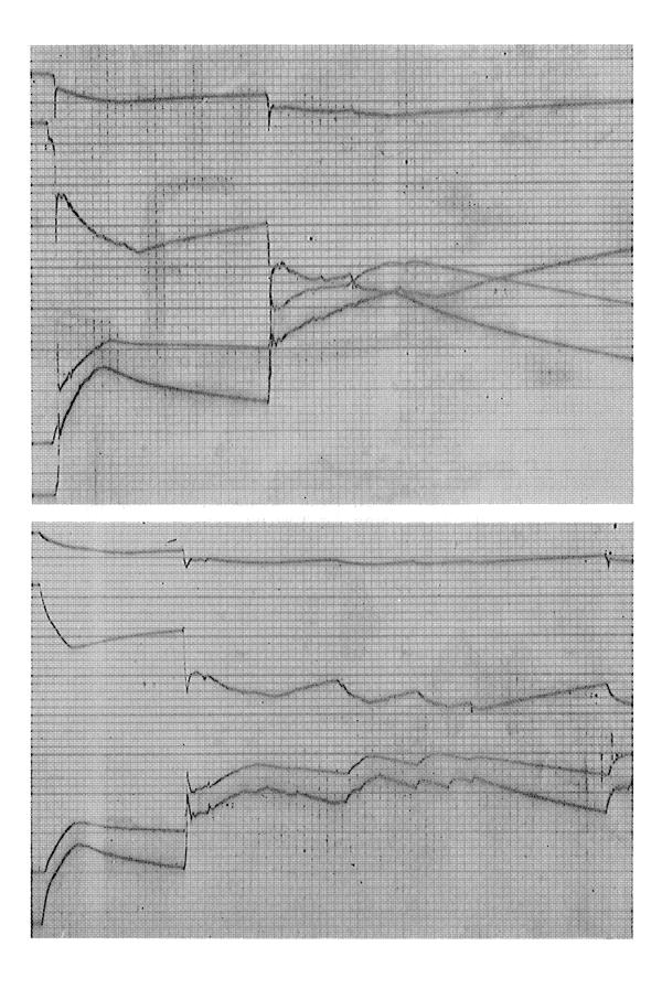
Figure 7. Three Typical Visicorder Records of Pressures on Face of Deckhouse During Typical Runs in Towing Tank
