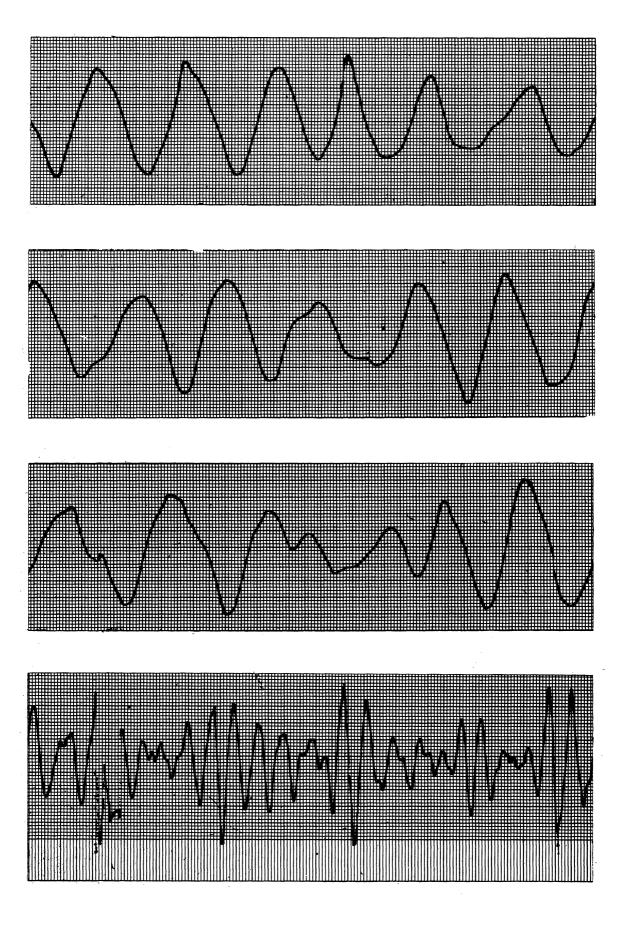
Figure 5. Two Typical Visicorder Records of Pressures on Face of Deckhouse During Typical Runs in Towing Tank
