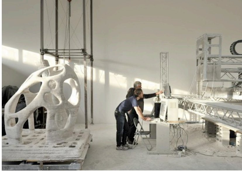
Figure 2: Enrico Dini and d-Shape Printer
