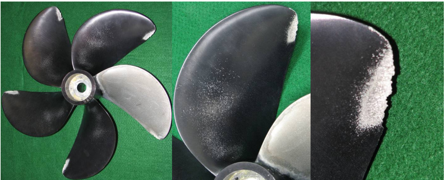
Figure 17: Cavitation Erosion Damage
