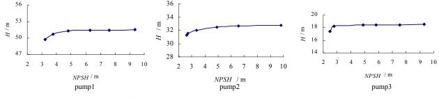
Figure 6 Cavitation performance prediction curve on design condition
