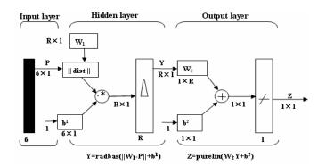
Figure 2 Architecture of RBF neural network
