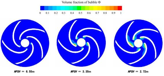
Fig.7 Volume distribution on middle section of impellers under different NPSH
