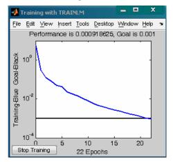
Figure 3 Curve of model error for BP network
