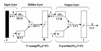
Figure 1 Architecture of BP neural network
