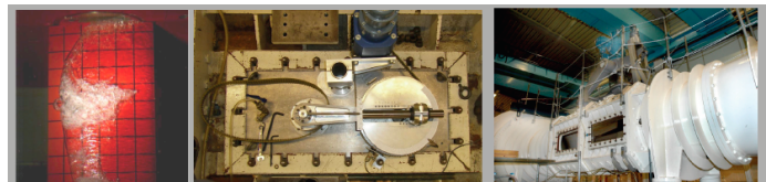
Figure 21 The foil, oscillation set up and the high-speed test section.
