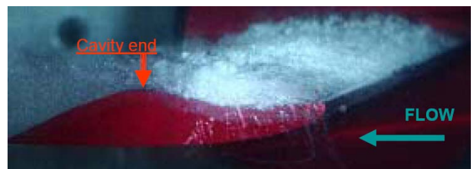
Figure 1: View of the hydrofoil OK2003 with ventilated cavity in the suction side concavity
