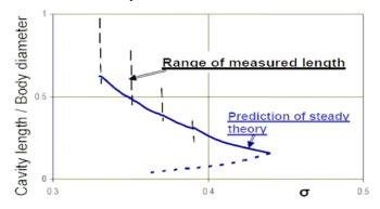
Figure 3: Comparison of observed (by Ceccio and Brennen, [9]) and computed (by Amromin, [6]) cavity lengths on the ITTC axisymmetric body (0.05m diameter).
