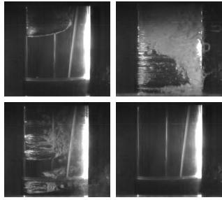
Figure 8. Stainless steel in weak water.  $\alpha = 4^{\circ}, \sigma/2\alpha = 4$ . View of cavitation at different stages in the oscillation cycle: Top Left: t = 0.142 period Top Right: t = 0.585 period Lower Left: t = 0.803 period Lower Right: Fully Wetted One period was equivalent to a time of 0.06 seconds. Flow is from left to right
