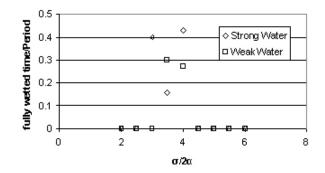
Figure 7. Fully wetted time on a stainless steel Cav 2003 hydrofoil at 4° angle of attack
