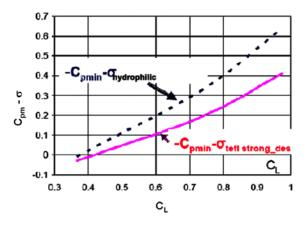
Figure 11 Calculation of -C<sub>pm</sub> - σ by Amromin [6]
