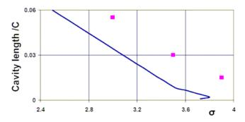
Figure 4: Comparison of computed and observed (after Amromin et al, [10]) cavity length on NACA-16009 hydrofoil with C=0.1m at 5 degree angle of attach in a narrow water tunnel.
