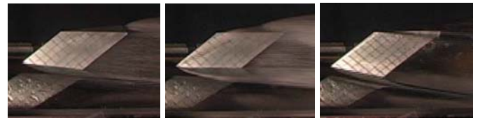
Figure 9: Different types of fin cavities during actuation. Left: small AoA, base cavity only. Middle: intermediate AoA, partial cavity from leading edge. Right: larger AoA, supercavity (clear) from leading edge.
