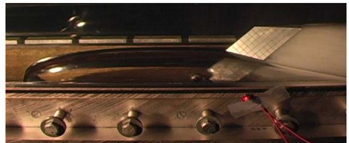
Figure 14: Stabilization and survival of marginal supercavity after slow control surface motion to target AoA.
