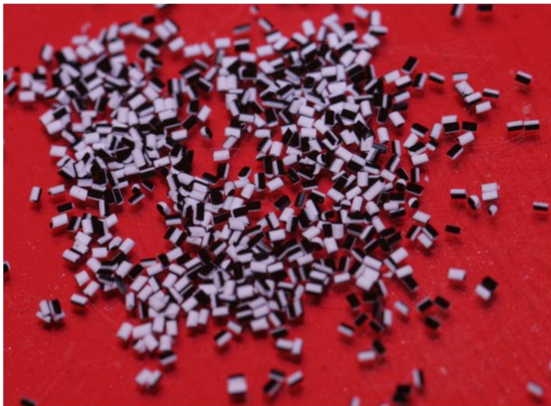
Figure 6.12 Digital photograph of optically visible microcylinders containing 5:100 wt. ratio of \text{TiO}_2 : PLGA in one compartment and 3:2:100 by wt. MNP:CB:PLGA in the black compartment. These cylinders were produced from fibers which were spun from solutions with greater viscosities (23:100 w/w PLGA in 95:5 Chloroform: DMF, 0.02 ml/h) using capillaries with larger diameters. Microcylinders have diameters of 250 \mu\text{m} and an aspect ratio of 1.
