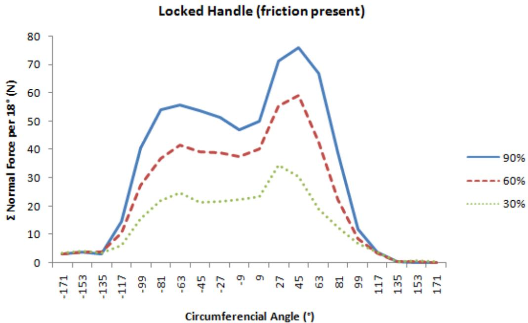
Figure 5.3.1 Integrated forces for each  $18^\circ$  band along long axis of handle for 30, 60 and 90% pull forces on the locked handle (friction present). The top of the handle is in the center of the graph ( $0^\circ$ ) and is the approximate location of the PIP joints. The bottom of the handle is at both ends of the graph ( $\pm 180^\circ$ ).
