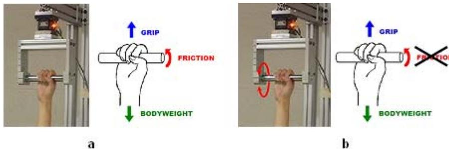
Figure 2.2.3 Breakaway handholds tested in Experiment 2. (a) Fixed 25mm horizontal cylinder. Friction resists the slipping of the hand. (b) Unconstrained 25mm horizontal cylinder. The cylinder can rotate about the long axis, nullifying the effect of friction that would resist slipping of the hand.
