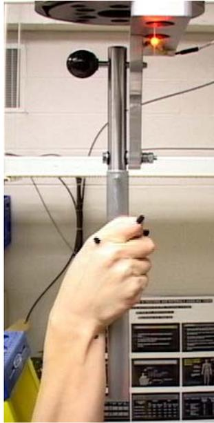
Figure 4.5.1 Typical wrist and finger posture on a vertical handhold. The wrist is ulnar deviated and individual finger's joints are flexed at different amounts: small finger flexed greatest, index finger least.
