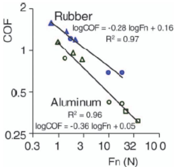
Figure 6.1.1 Friction coefficient as a function of normal force for rubber (filled symbols) and for aluminum (unfilled symbols) from three studies ( $\Delta$ ), Seo et al. accepted; (o), the present study; ( $\square$ ), Buchholz et al. 1988) in log scales. COF = coefficient of friction. (From Seo & Armstrong, 2009)
