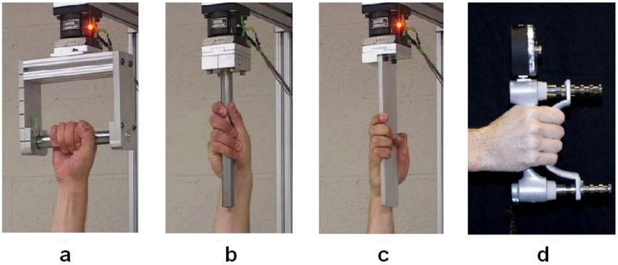
Figure 2.2.2 Handholds tested. (a) 25mm diameter horizontal cylinder (Experiment 1 and 2) (b) 25mm vertical cylinder (Experiment 1 only) (c) 64mm x 10mm vertical plate (Experiment 1 only) (d) Jamar grip dynamometer in position 2 (Experiment 1 and 2).
