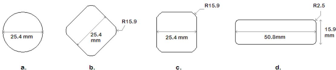
Figure 3.2.1 Handle cross-sections. (a) “cylinder”: circle of diameter 25.4mm (b) “diamond”: 25.4mm square rotated 45° (c) “square”: 25.4mm square (d) “rectangle”: 50.8x15.9 mm rectangle. R=corner radius of curvature in mm.
