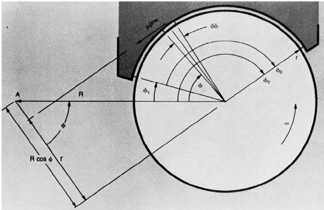
Figure 6.1.3 Geometry for calculating the moment due to friction about pivot about point A. From: Orthwein (2004).
