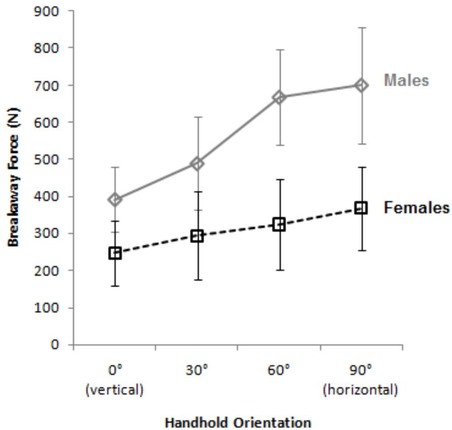
Figure 4.4.1 Mean breakaway strength (N) by orientation for male and female subjects. Strength decreases for handle orientations from horizontal to vertical.
