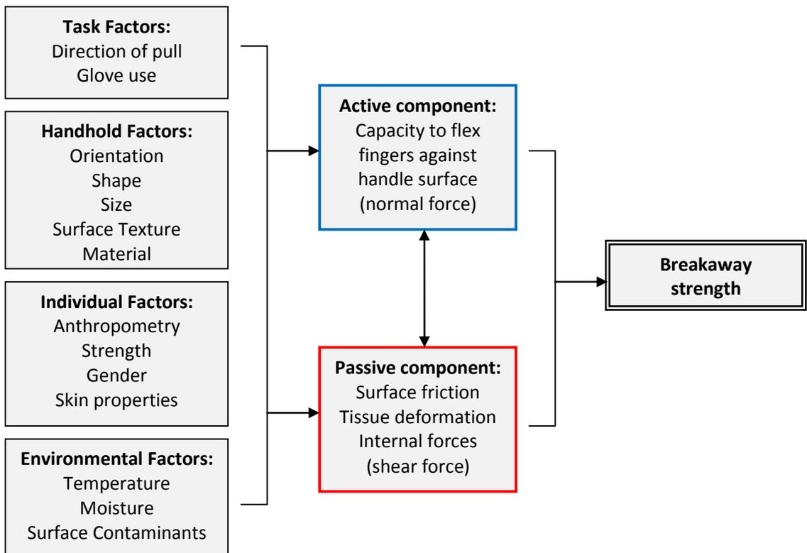
Figure 6.1.4 High-level overview of factors affecting breakaway strength. Hand/handhold coupling is comprised of both active and passive components that influence each other.
