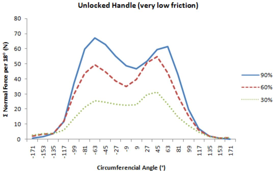
Figure 5.3.2 Integrated forces for each 18° band along long axis of handle for 30, 60 and 90% pull forces on the unlocked handle (very low friction). The top of the handle is in the center of the graph (0°) and the bottom of the handle is at both ends of the graph ( $\pm 180^\circ$ ).
