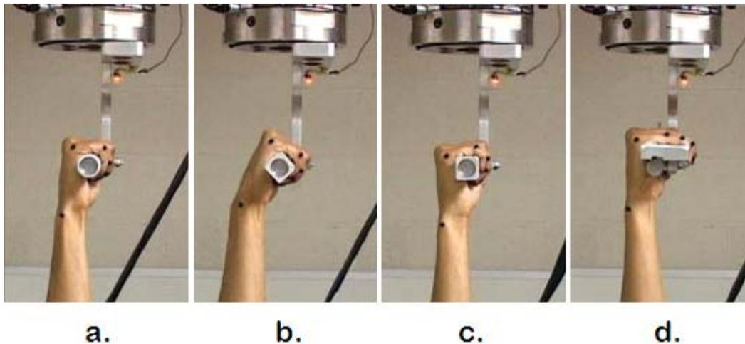
Figure 3.2.2 Initial subject hand posture when performing breakaway strength measurements. Small markers indicate finger joints. For the cylinder, no starting hand position was specified. For other shapes, subjects placed the palmar skin crease of the finger MCP joint on the top corner of the (b) diamond or closest corner of the (c) square or (d) rectangle. As loading increases the skin can translate slightly with respect to the underlying bones.
