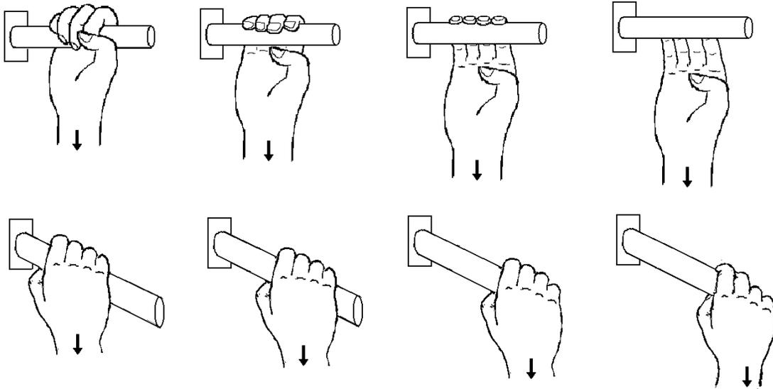
Figure 4.3.3 Types of coupling failures. In the horizontal handhold orientation (top row), the fingers must be forced open under the vertical load. The fingers slide over the circumference of the cylinder as fingers are forced open (coded ‘+1’). As the handhold orientation moves from horizontal to vertical (bottom row), the fingers may not be forced open and the vertical load causes the hand to slide down the long axis of the handle and off the end (coded ‘-1’).
