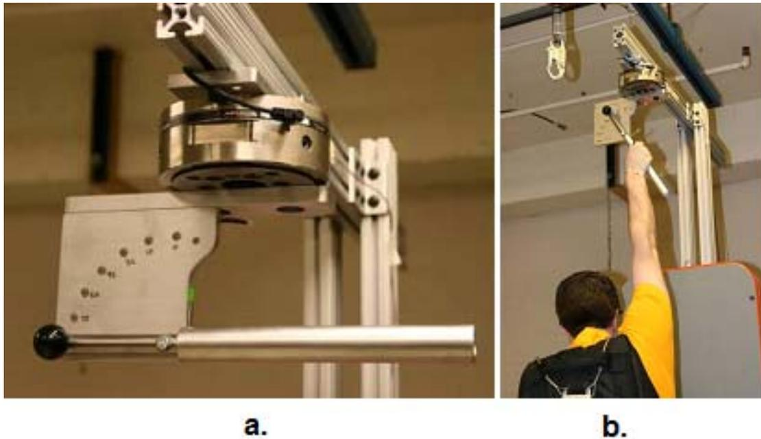
Figure 4.3.1 Experimental apparatus. a) An adjustable handle was attached to a 6-axis load cell. The handle could be adjusted to be oriented in 15° increments between horizontal and vertical. Different diameter metal cylinders can be easily interchanged. b) Subject position during breakaway trials.
