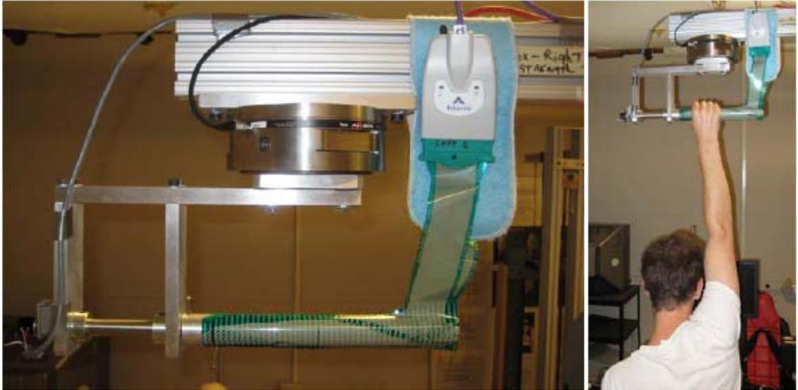
Figure 5.2.1 Experimental setup. A cylindrical handle is attached to a six-axis load cell and a pressure sensitive mesh is wrapped around the surface of the handle (left). Subjects grasped the overhead handle and either squeezed or pulled downward on the handle while watching a computer screen to match a desired force (right).
