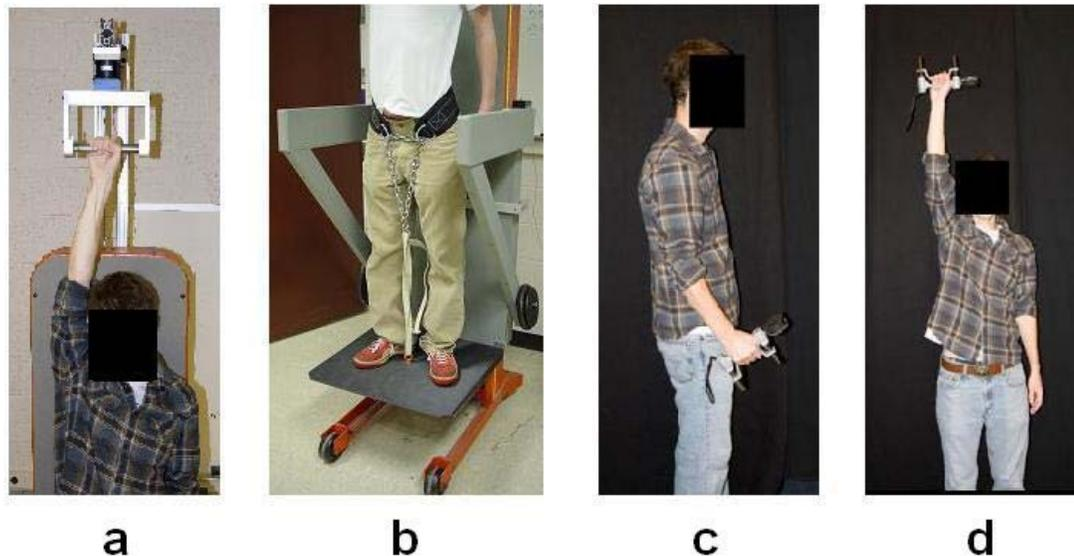
Figure 2.2.1 Experimental setup. (a) Subjects stand on a platform and are lowered while grasping an instrumented, fixed-overhead handle. (b) Subjects are secured to the weighted platform by a weightlifter's dipping belt so they cannot lift themselves off of the platform and always move up or down with it. (c) Subject position for isometric grip strength measurements (Experiment 1 and 2). (d) Subject position for additional isometric grip strength measurement (Experiment 2 only).
