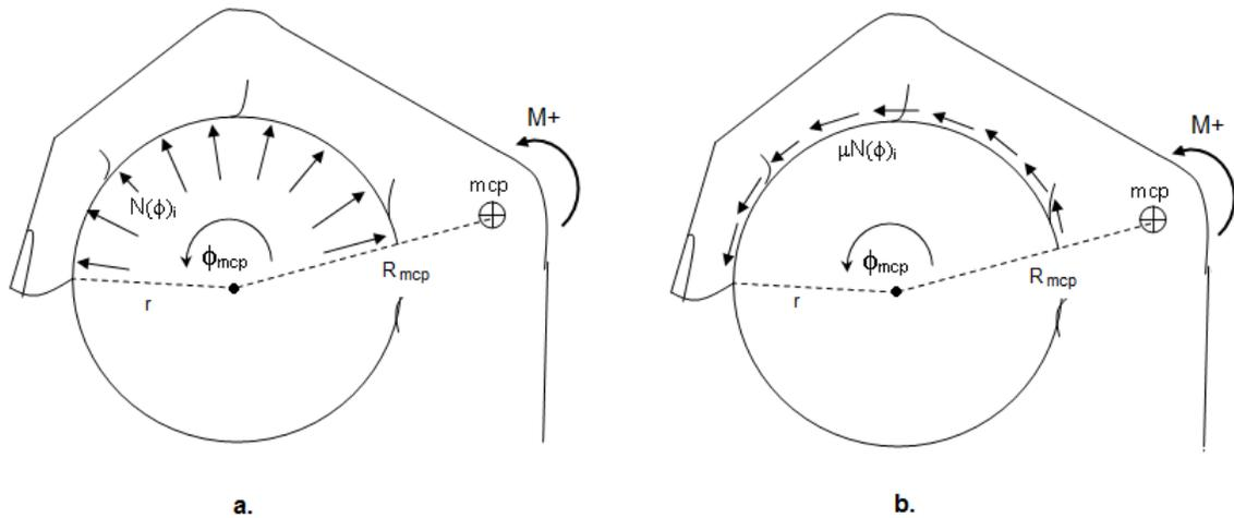
Figure 5.3.4 Illustration of parameters used to calculate resultant joint torque for the MCP joint. Normal forces (a) and frictional forces (b) over the contact arc of the finger cause a resultant moment about the MCP joint that must be balanced by internal flexion moment in order to maintain static equilibrium about the MCP joint. By definition, the joint center is at  $\varphi=0^\circ$ .
