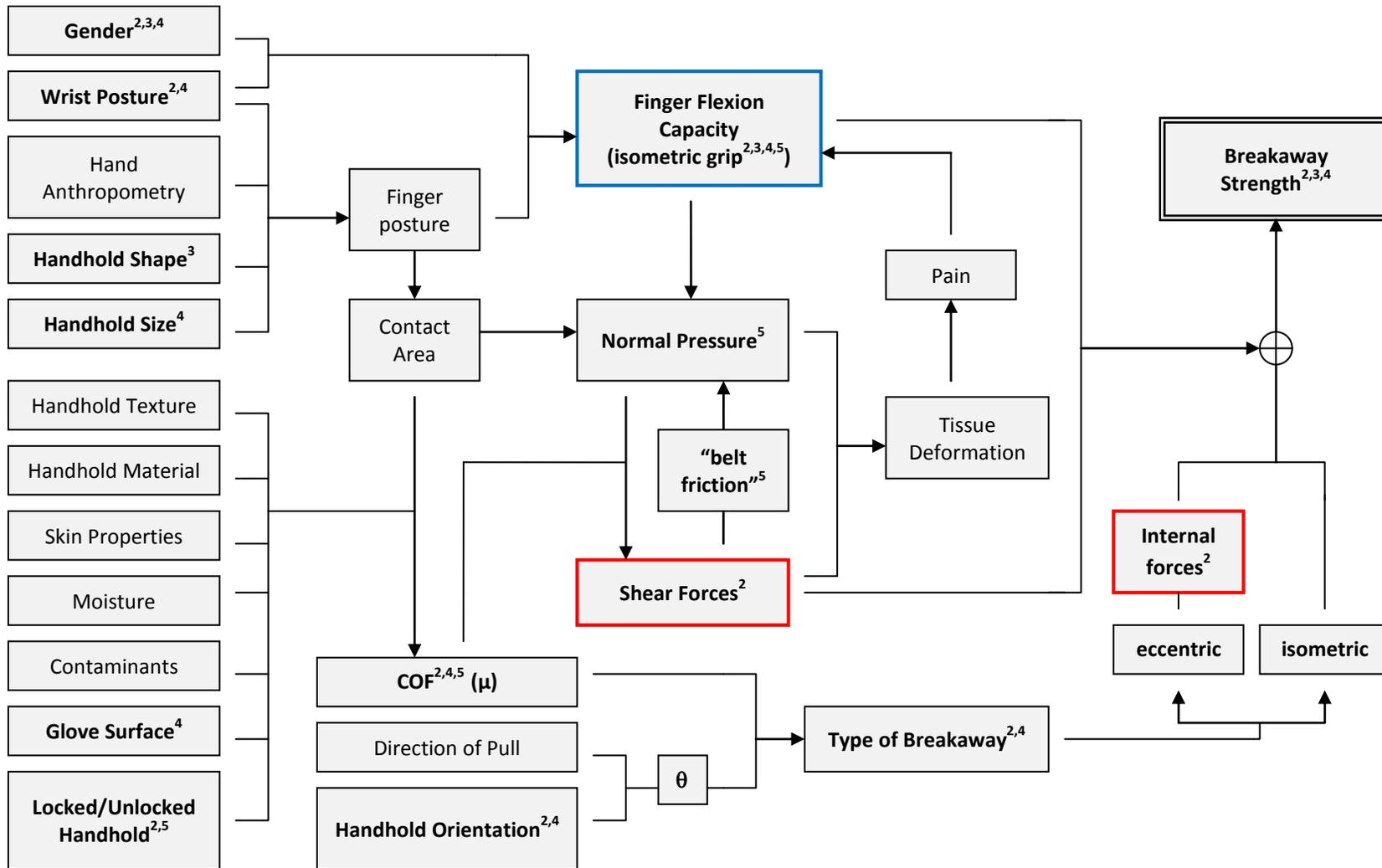
Figure 6.1.5 Schematic of factors influencing breakaway strength. Items in bold are addressed either directly or indirectly by experiments presented in this dissertation (Chapter numbers indicated by superscripts). Several factors (left side) act to generally affect either the capacity to flex the fingers (active) or the coefficient of friction (passive). Both active and passive components act to influence each other (center area) and total breakaway strength (right side).
