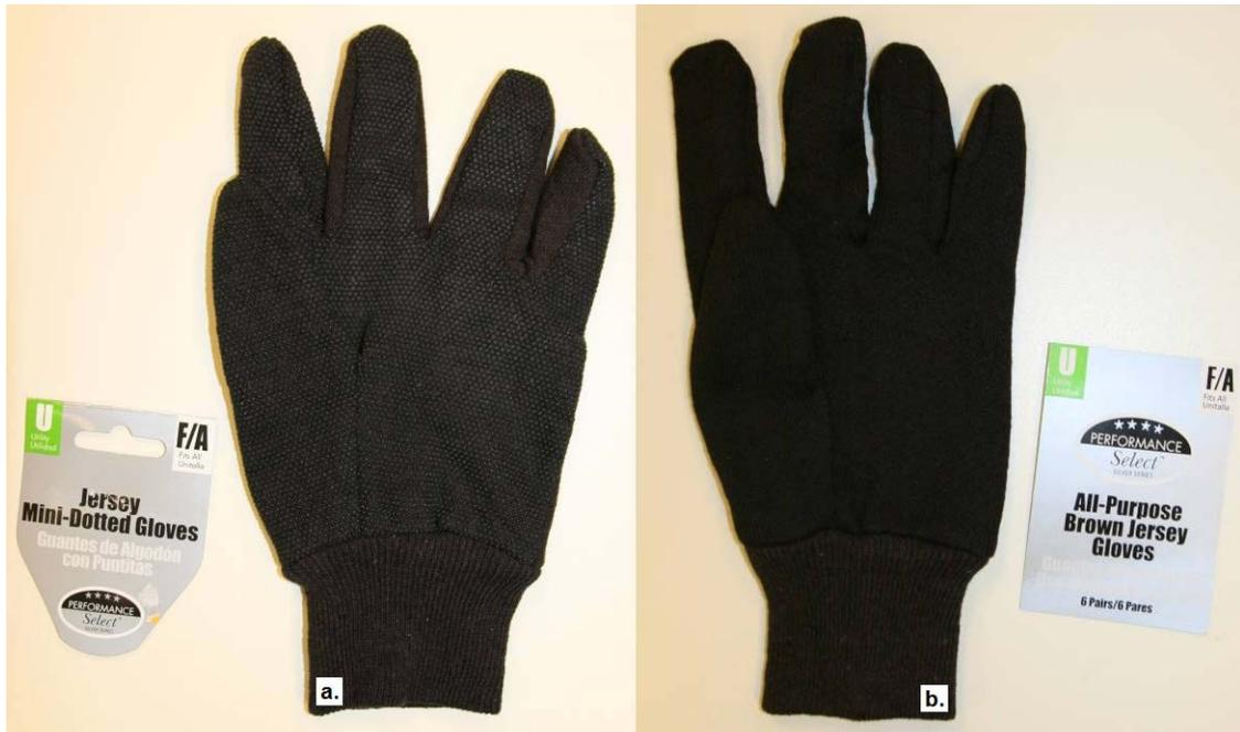
Figure 4.3.2 Gloves tested in Experiment 2 (non-dominant hand). (a) PVC dotted “high-friction” glove,  $\mu \approx 0.70$  (b) plain jersey cotton “low-friction” glove,  $\mu \approx 0.27$ . Frictional characteristics of the gloves were estimated by measuring the force at onset of movement required to pull a 1 kg aluminum plate over a gloved hand with fingers flat and palm supine.
