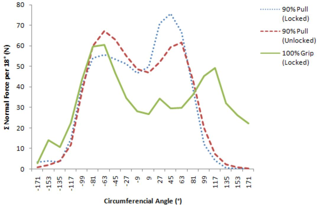
Figure 5.3.3 Integrated forces for each 18° band along long axis of handle for 90% pull forces on the locked and unlocked handles and 100% gripping effort (no pull force).
