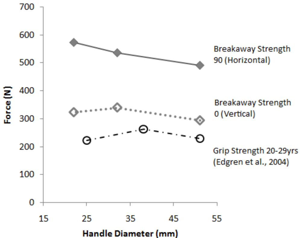
Figure 4.5.2 Mean breakaway strength vs. handhold size for horizontal and vertical handholds (Experiment 1) and voluntary isometric grip strength vs. handle size for subjects aged 20-29 from Edgren et al.. (2004). Males and females are pooled. Strength was consistently least for the largest cylinder. Strength was greatest for the 32 mm diameter handle in the vertical orientation, while strength was greatest for the smallest diameter in the horizontal orientation.
