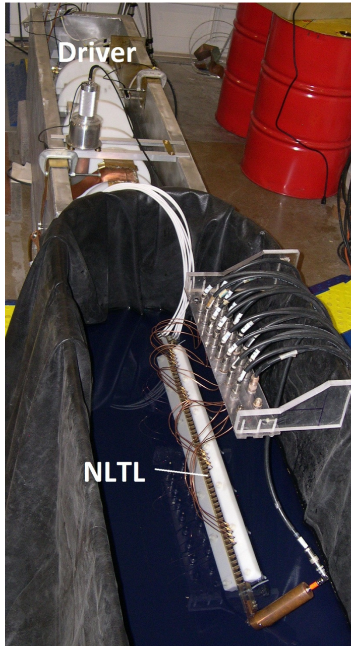
Figure 4-17. Driver oil tank at top connected with eight 50 \Omega cables to NLTL in adjacent oil tank at bottom.
