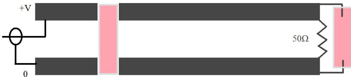
Figure 5-4. Diagram showing the two possible test tube locations for electroporation. Note that only a single tube, either conductive (right test tube) or capacitive connection (left test tube), would be present during a given shot.
