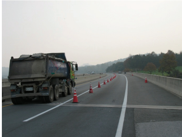
Figure 7.2 Vehicle-bridge interaction testing with a 20.9-ton test truck on the Yeondae Bridge.
