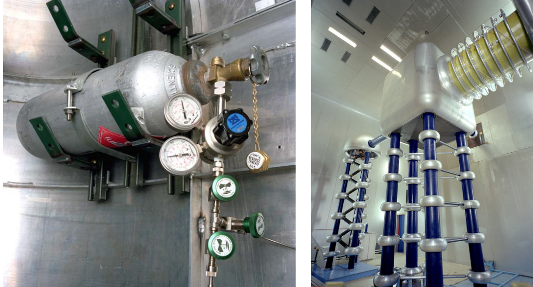
Figure 3.2: The hydrogen gas from which the accelerated protons are derived (left), and the Cockcroft-Walton accelerator which employs a 750 kV static electric field (right).
