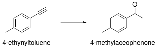
Figure 5.3: 4-ethynyltoluene hydrates to form 4-methylacetophenone.
