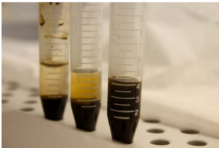
Figure 2.32: Colloidal stability of magnetite nanoparticles in water after 18 hours. (A) sodium citrate coated MNP, (B) gum arabic coated MNP, and (C) non-coated MNP
