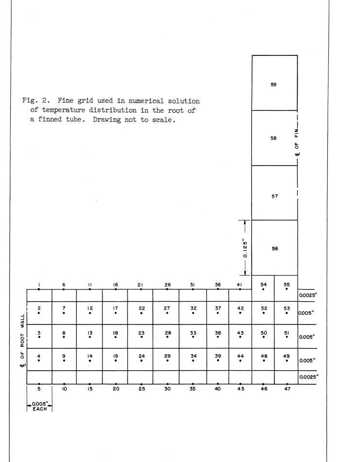
steady-state heat transfer conditions there will be no accumulation of thermal energy in any one grid. Therefore, the rate of heat transfer to the grid under consideration is equal to the rate of heat transfer from the grid.
