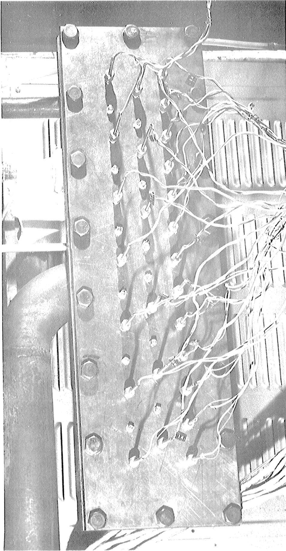
Fig. 2 Water Exit Header of Experimental Unit Showing Cover Plate with Locations for 39 Thermocouples
