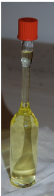
Figure 6.2: Uranium complex dissolved in liquid scintillator, showing the yellow coloration characteristic of uranyl oxides.
