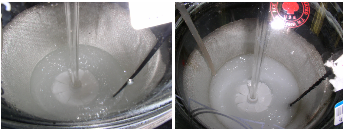
Figure 3.2: Left: Sodium fluoride/oleic acid solution before the addition of cerium nitrate. Stirrer is visible in center, thermometer is visible on right. Right: Sodium fluoride/oleic acid solution after the addition of cerium nitrate. Solution has turned white due to the formation of oleic-capped cerium fluoride particles.
