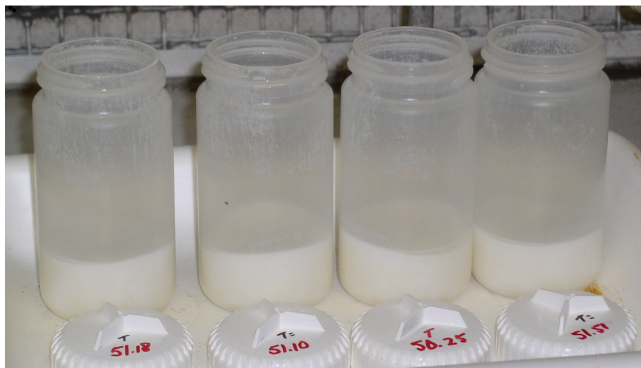
Figure 3.5: \text{CeF}_3 nanoparticles drying in the hood after washing
