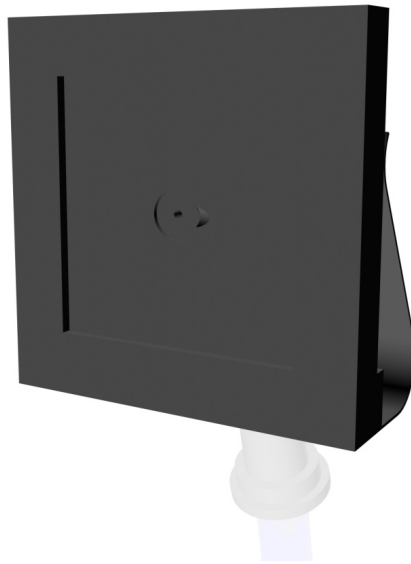
Figure 4.5: Rendering of the optically stimulated luminescence (OSL) reader sample holder assembly. The sample is placed in the center of this plate and the vacuum line attaches to the small hole in the center, from behind.
