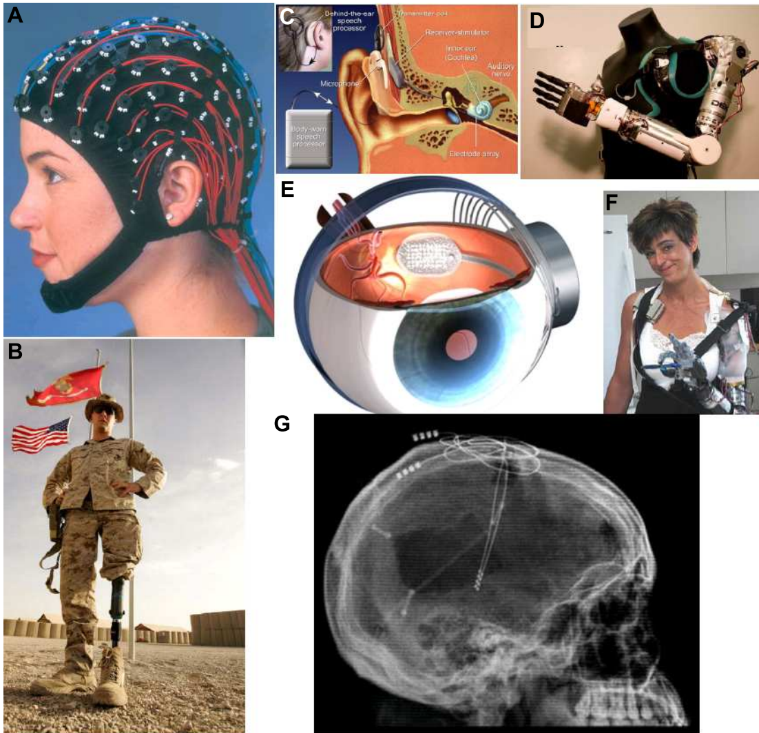
Figure 1.1: Examples of prosthetic devices. (A) EEG P300 speller for locked-in patients. (B) Prosthetic leg with a controlled knee joint. (C) Cochlear Implant. (D) New 22 degrees of freedom prosthetic arm. (E) Second Sight retinal implant. (F) Prosthetic arm being used. (G) Medtronic deep brain stimulator. (Images were provided by DARPA, Medtronic, and Second Sight.)
