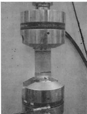
Figure 1: Uniaxial tension testing setup
