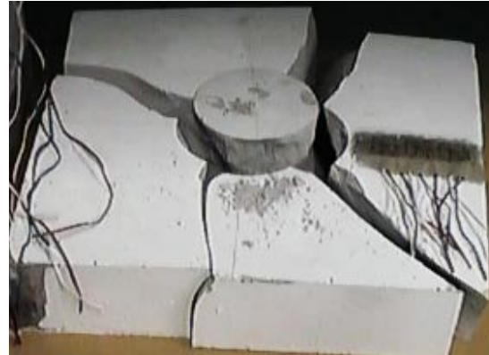
Fig. 3: Failed Mortar Specimen
