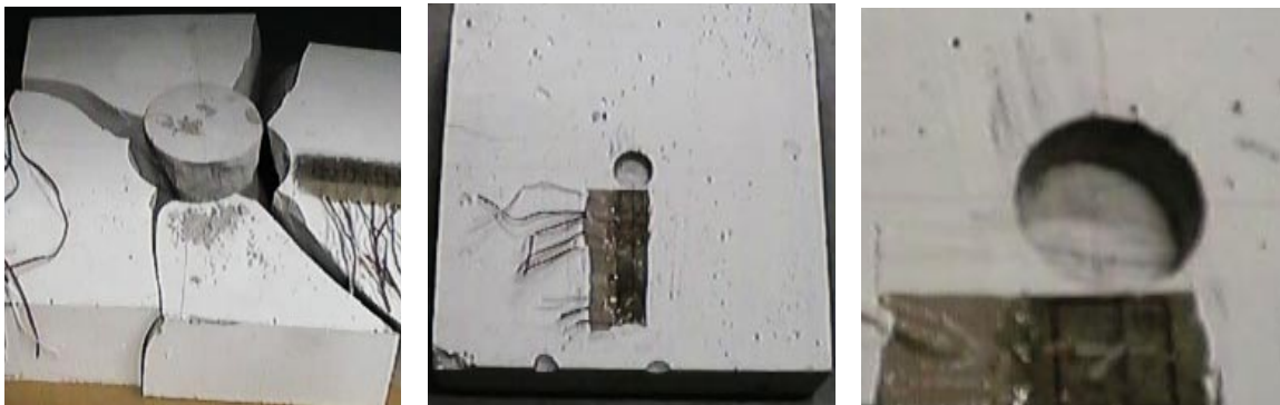
Figure 9: Failure Modes of (a) Mortar Slab, (b) PVA-ECC Slab and (c) Closeup View Near Indent
