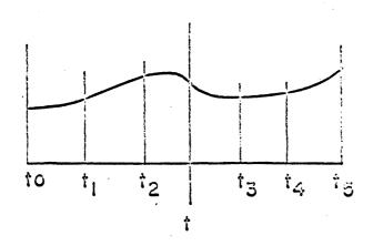
Figure 4.3.2 Since  $t_2 < t < t_3$ , the m.l.s. decomposition process does not alter the break points  $t_1$  and  $t_2$ .
