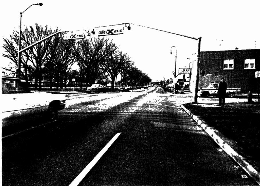
FIGURE 2-18 TYPICAL UNSIGNALIZED LOCATION WITH MAST ARMS
