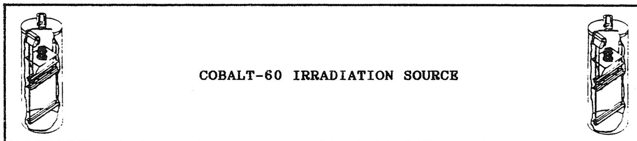
The cobalt-60 source of approximately 10,000 curies is available for gamma irradiations. Typical applications include sterilization of bone and cartilage for human grafts and transplants; sterilization of animal food for germ-free animal colonies; studies of radiation effects on mutation of cells, chemical systems, electronic and reactor components, food, seeds, and plants.
