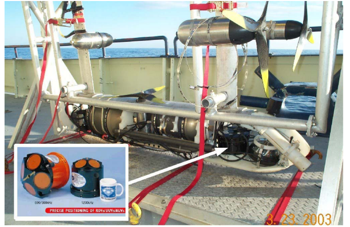
Fig. 4. A RD Instruments 1200 kHz Workhorse Navigator DVL is shown in-situ on the bottom hull of the SeaBED AUV (outer hydrodynamic shell removed).
