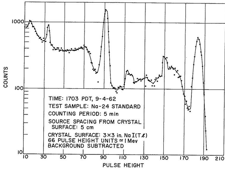
Fig. 14. Pulse height spectrum, Na-24 standard
