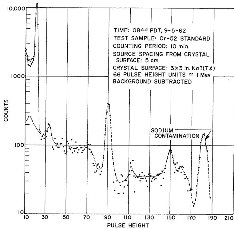
Fig. 22. Pulse height spectrum, Cr-52 standard
