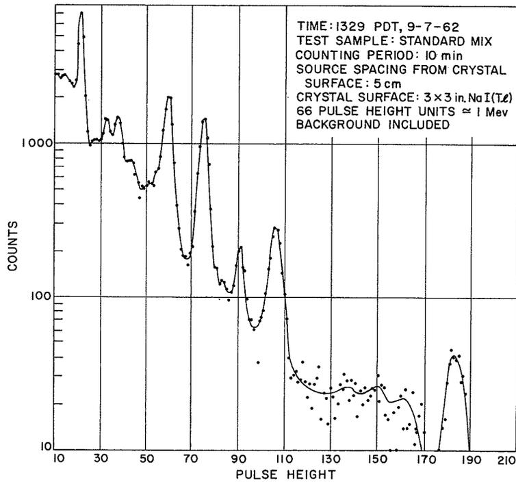
Fig. 11. Pulse height spectrum, standard mix, 1329 PDT, 9-7-62
