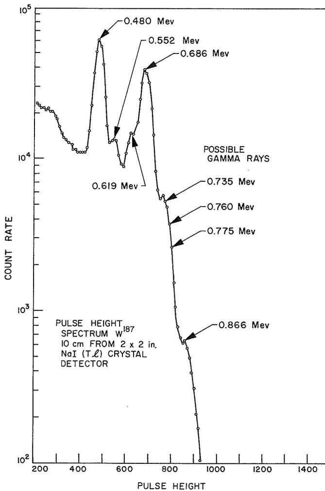
Fig. 2. Pulse height spectrum,  $W^{187}$
