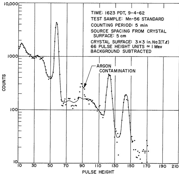
Fig. 17. Pulse height spectrum, Mn-56 standard
