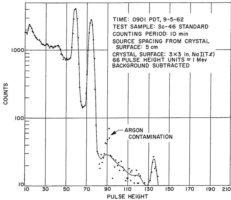
Fig. 18. Pulse height spectrum, Sc-46 standard
