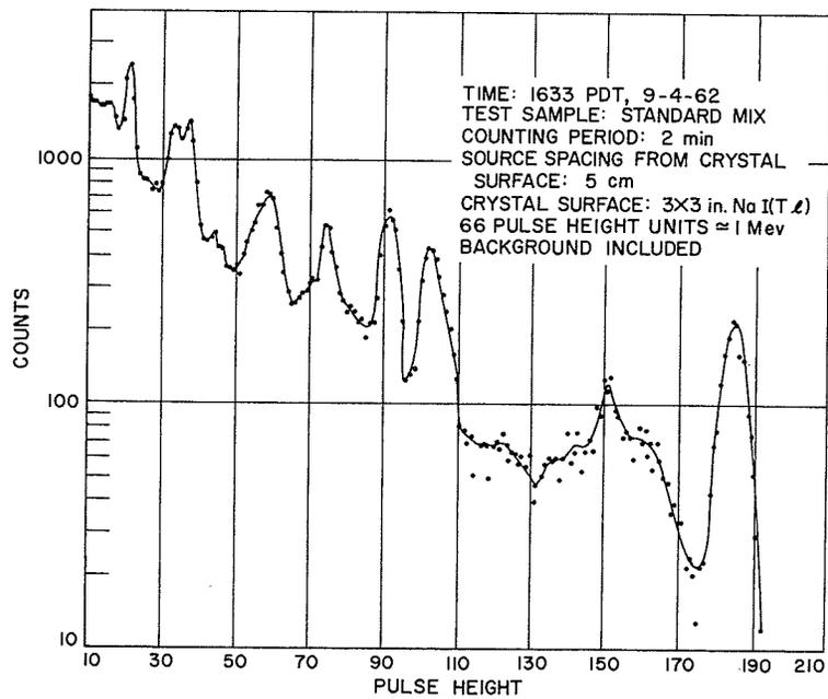
**Fig. 7. Pulse height spectrum, standard mix, 1633 PDT, 9-4-62**
