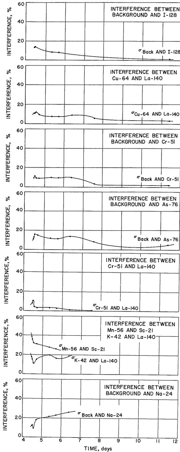
Fig. 25. Interference between various component spectra
