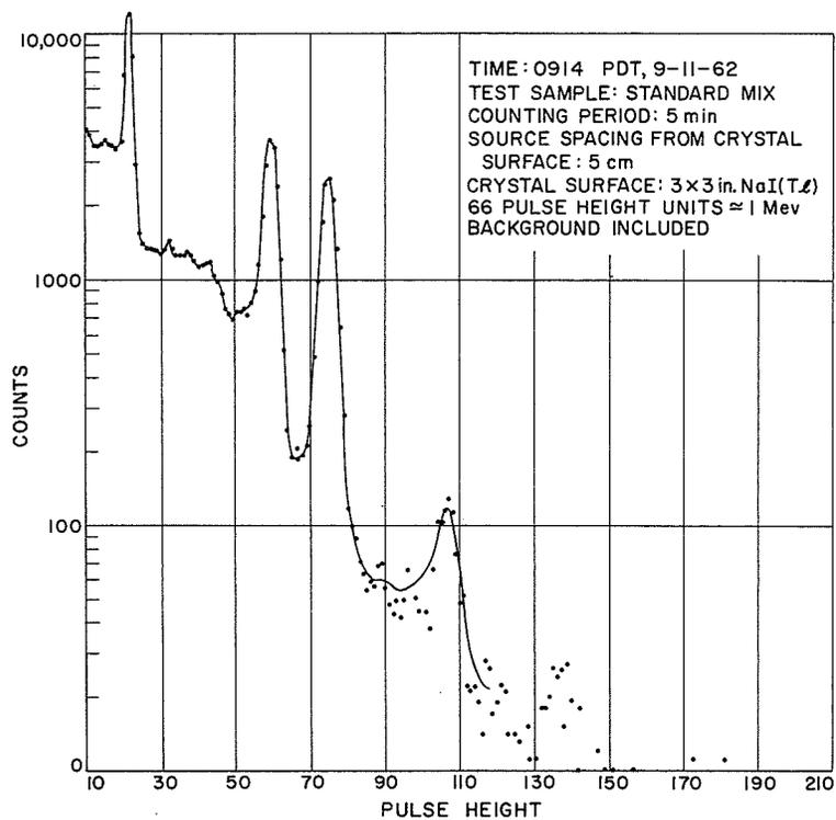
**Fig. 12. Pulse height spectrum, standard mix,
