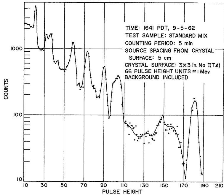
**Fig. 9. Pulse height spectrum, standard mix, 1641 PDT, 9-5-62**
