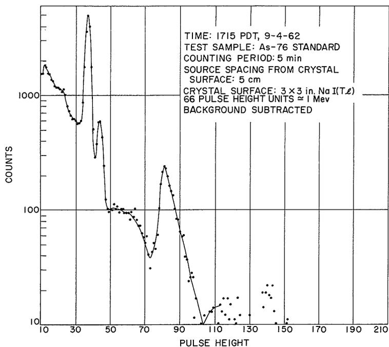
Fig. 20. Pulse height spectrum, As-76 standard
