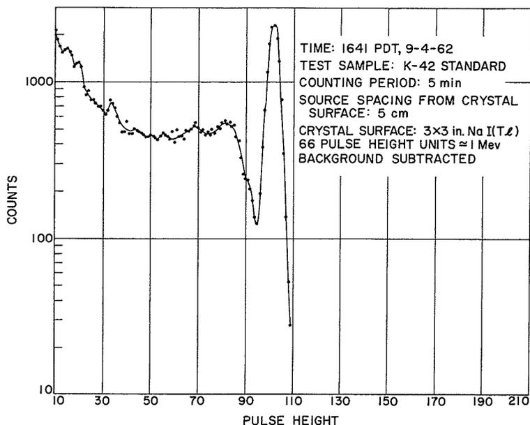
Fig. 16. Pulse height spectrum, K-42 standard
