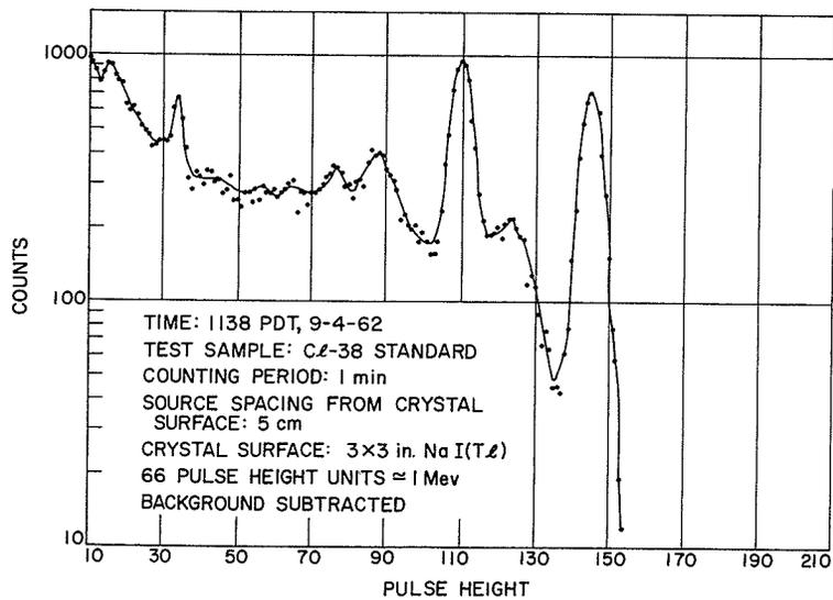
Fig. 15. Pulse height spectrum, Cl-38 standard
