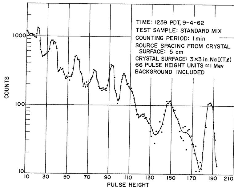
**Fig. 6. Pulse height spectrum, standard mix, 1259 PDT, 9-4-62**
