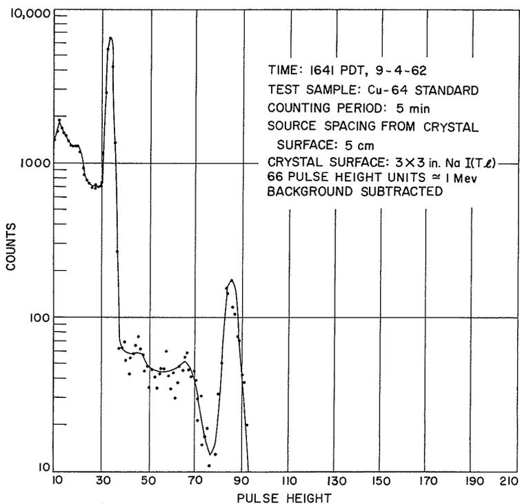
Fig. 21. Pulse height spectrum, Cu-64 standard
