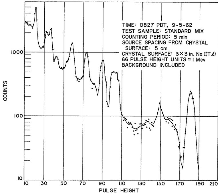
**Fig. 8. Pulse height spectrum, standard mix, 0827 PDT, 9-5-62**
