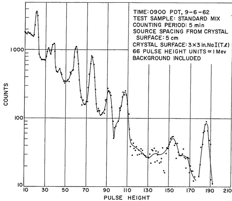
Fig. 10. Pulse height spectrum, standard mix, 0900 PDT, 9-6-62
