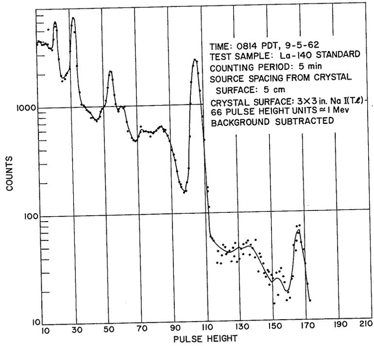
Fig. 24. Pulse height spectrum, La-140 standard
