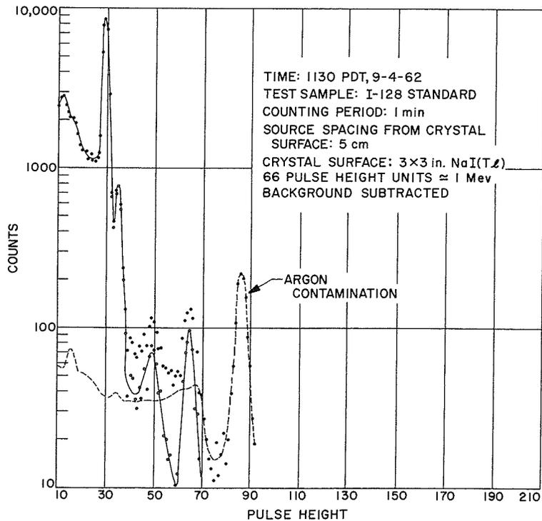
Fig. 23. Pulse height spectrum, I-128 standard
