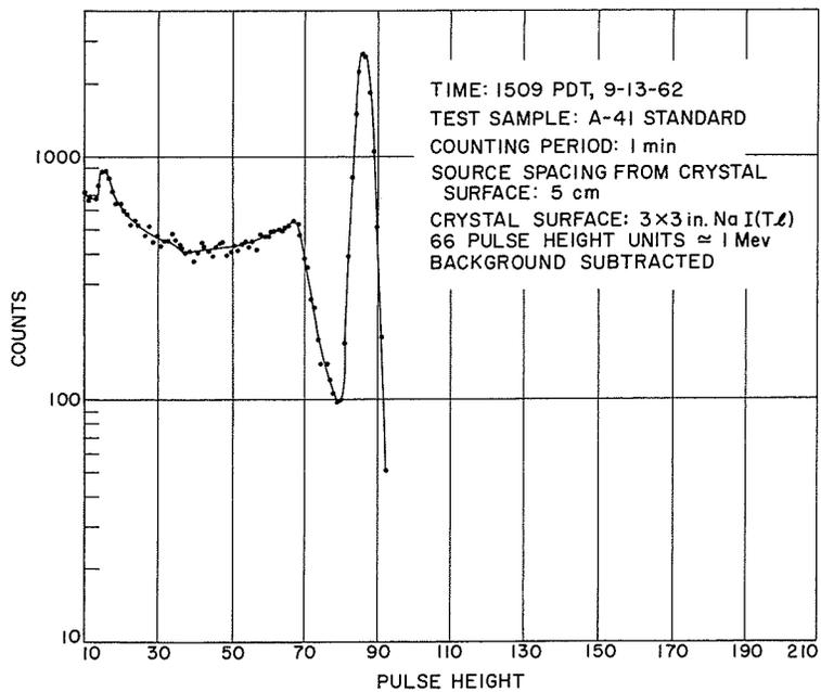
Fig. 19. Pulse height spectrum, A-41 standard
