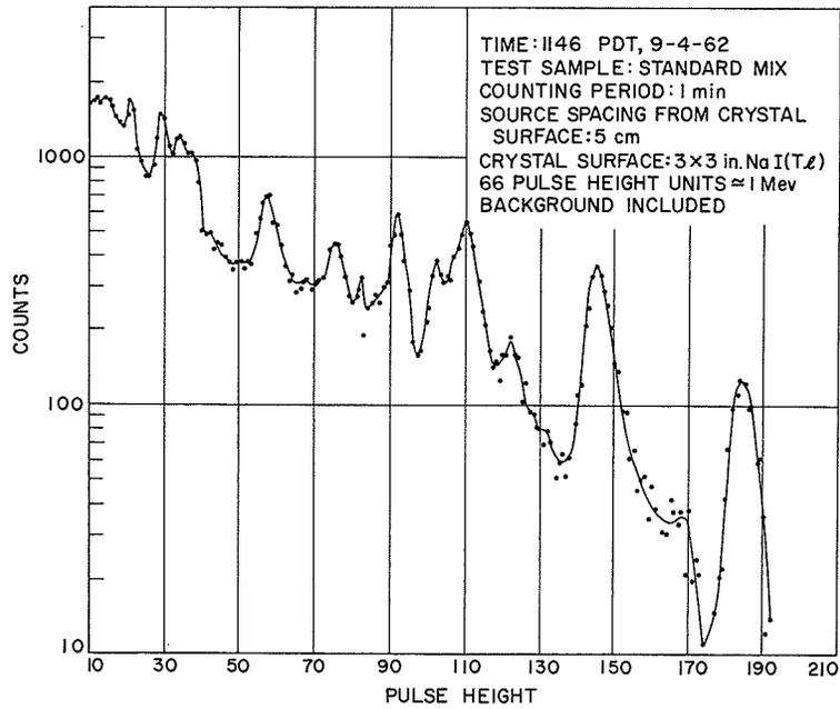
Fig. 5. Pulse height spectrum, standard mix, 1146 PDT, 9-4-62
