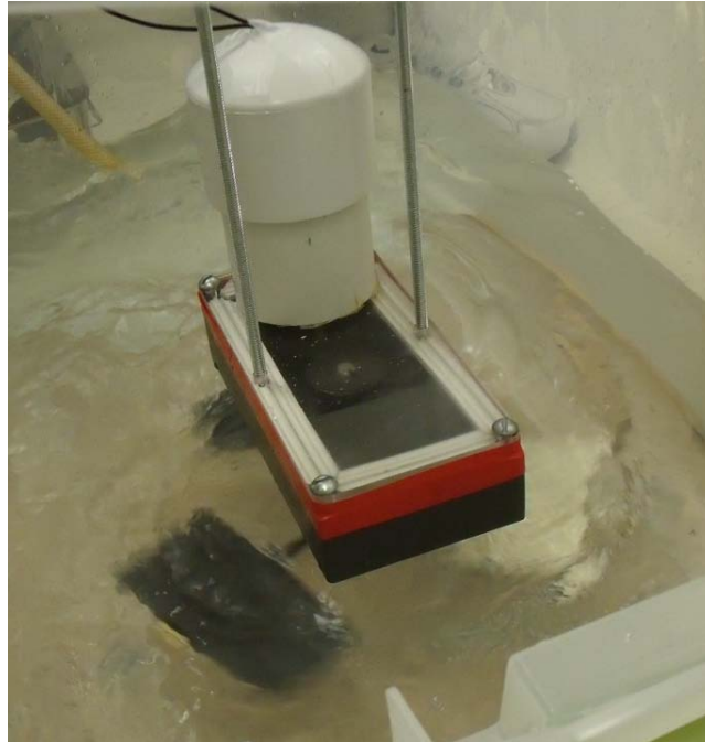
Figure 30: The hydrofoil shoe running in the test rig
